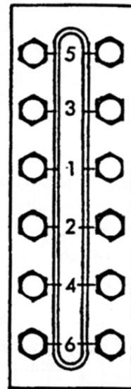
**CAUTION:** Bolts or nuts should not be tightened unless the gage is isolated from the vessel and the gage is vented to the atmosphere.
