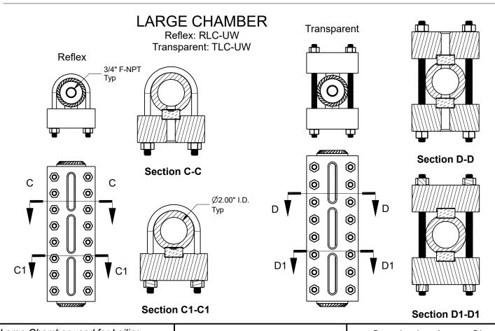
Large Chamber used for boiling hydrocarbons to stabilize view and allow accurate level reading
