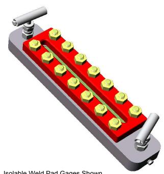
Isolable Weld Pad Gages Shown are Non-Automatic. Valves do not have ball check shut-off feature & will not stop leakage of the contained fluid in the event of accidental gage glass breakage (except by minimal closing of the valves).
