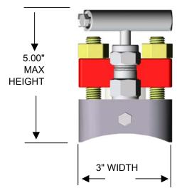
Pad curved to fit pipe or flat as required
