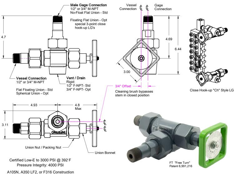
Stem packing isolates valve workings from process (salt water, H2S etc) <u>FT "Free Turn" Advantages</u>
